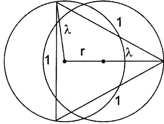
FIG. 2. External geometry for three sphere centers just to fit on the boundary of a  $(r, \lambda)$  double cavity. The three spheres are in mutual contact, and are coplanar with the centers of the two  $\lambda$  spheres comprising the double cavity.
