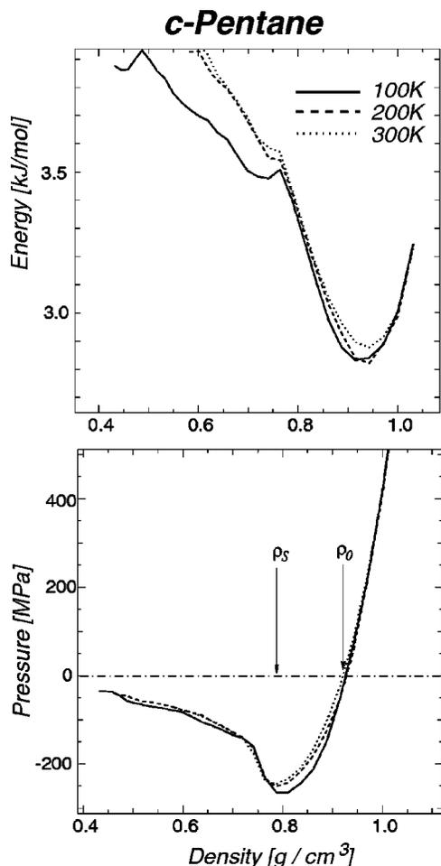
FIG. 3. Potential energy (top) and pressure (bottom) of inherent structures obtained from liquid cyclopentane at various temperatures as a function of density.  $\rho_S$  (Sastry density) is the limit of mechanical stability of the inherent structures with respect to isotropic tension;  $\rho_0$  corresponds to the minimum inherent structure energy and fulfills a zero-pressure condition.
