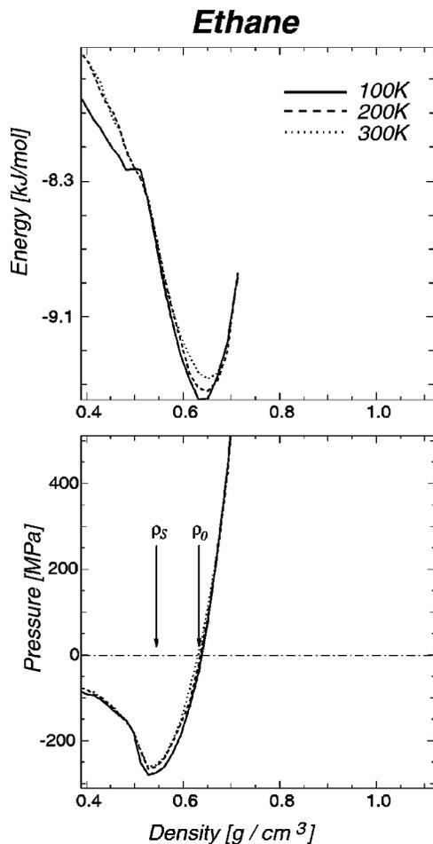
FIG. 1. Potential energy (top) and pressure (bottom) of inherent structures obtained from liquid ethane at various temperatures as a function of density.  $\rho_S$  (Sastry density) is the limit of mechanical stability of the inherent structures with respect to isotropic tension;  $\rho_0$  corresponds to the minimum inherent structure energy and fulfills a zero-pressure condition.
