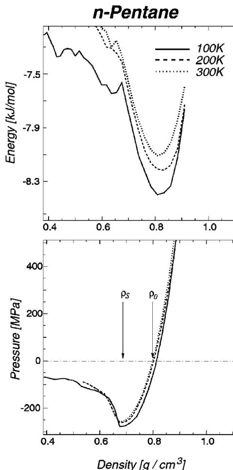
FIG. 2. Potential energy (top) and pressure (bottom) of inherent structures obtained from liquid pentane at various temperatures as a function of density.  $\rho_S$  (Sastry density) is the limit of mechanical stability of the inherent structures with respect to isotropic tension;  $\rho_0$  corresponds to the minimum inherent structure energy and fulfills a zero-pressure condition.
